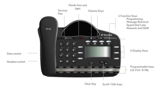
This diagram illustrates the V16 phone which has 16 programmable keys
